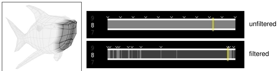
Figure 2.4: Shark model with snout highlighted and the corresponding timeline with and without filtering. To focus on edits affecting only specific regions of the mesh, the viewer highlights the areas of interest, and the timeline is filtered to show the clusters that modify these areas.
